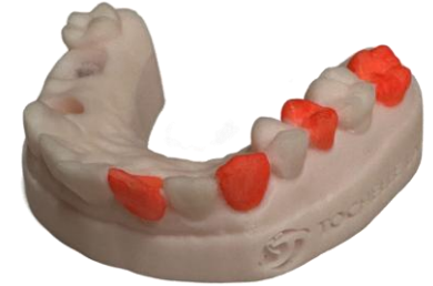
The teeth used in the CAD model were printed and coloured, to allow for easy differentiation of individual teeth in the captured images.
